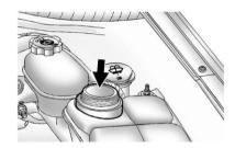
Fill the coolant surge tank with the proper DEX-COOL coolant mixture until the level inside stabilizes at the FULL COLD mark on the front of the surge tank.
